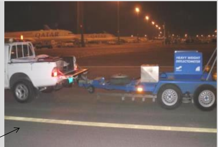
Deflectometric surveys with HWD device
